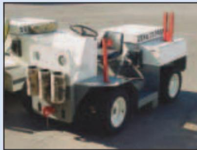
PSI Mdl. X3-WT Aircraft Tug, 5,000 Lb. DBP, Auto Trans., 4 Cyl. Chrysler Engine
