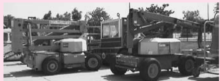
Genie Mdl. Z-45/22 Electric Boom Lift, Work Load 500 Lb., Platform Height 45' Genie Mdl. Z-30/20 HD Electric Boom Lift, Max Load 500 Lbs., Platform Height 31'
