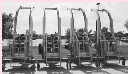
(4 ea) Electric Personal Lifts For Riveting Top of Fuselage-Challenger Aircraft
