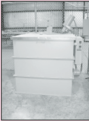
L&L Special Furnace Co. Industrial Quench Tank Mdl. QT3648-FB24-01-G508-240R31H-H99, 240 Volt, Max. Temp 200F w/ Agitator
