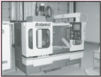
Bridgeport Interact CT520 CNC Vertical Maching Center w/Hudenhain TNC155 Control Panel
