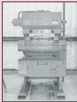
Wysong Mdl. H2052 Press Brake, 13 Ton Mid Stroke, 20 Tons Near Bottom 2.5" Stroke w/Several Misc. Dyes, S/N hp612-229
