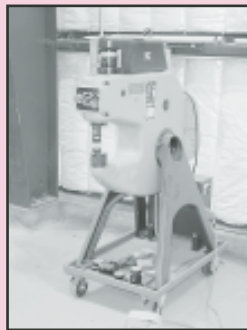
Eckold Mdl. KF 330 Piccolo Sheet Metal Shrinker Stretcher, S/N 5048, 12" Throat w/Variou Shrinking and Stretching Heads
