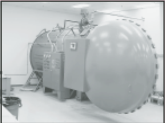
Melco Autoclave, 10' OD x 40' L, 8' ID x 36' D, Max WP 290 PSI @700 F, S/N 2088, Built 1986, Shell Thickness 1.00", Head Thickness 96", National BD 263 w/New Taricco Corp Thermal Control System Version 1.82. Unit was Refurbished in 1999 by Taricco Corp.
