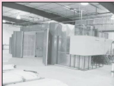
Spray Systems Inc. Paint Booth, 20' W x 12' T x 34' D w/Banza Mdl. B-2000 Air Mgmt. System Controls, Heats Up To 170F w/ Explosion Proof Lighting and Sprinkler System, Bi-Fold Doors Various Control Surface Balancing Fixtures
