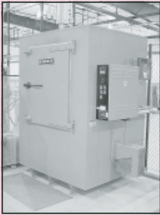
Grieve Mdl. HB-1250, 60 Watt High Input, 230 Volt, 3 PH, Max 1250 F, S/N 520040 w/ A Partoow M/C-6000 Digital Readout & Honeywell DR4300 Circular Chart Recorder
