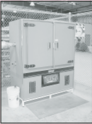
Blue M Electric Oven Mdl. DC-1406-B, 208 Volts, 60 Htz, 1 PH, Heater Capacity 6.8 KW w/A Type J and Stat 1900 Controllers, Up to 750 F and BM-7000 Circular Chart Recorder, S/N V24E-215951-VEDDY
