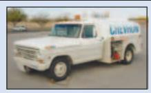
1968 Ford F-350 AV-Gas Truck, 750 Gallon Tank, Single Pump and Meter, 10 GPM Flow, Top and Bottom Load, 6 Cyl. Engine
