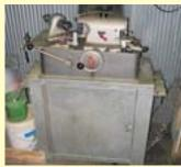
Sioux Mdl. 645 Wet Valve Facing Machine w/ Rocker Arm Attach. Sioux Valve Seat Driver, Mdl. 172 w/Pilots and
