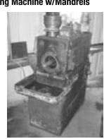
Barnesdrill Cylinder Barrel Lapping Machine
