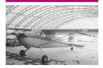
Cessna 140 Aircraft N-2318 V S/N 14554 1734 Hrs. Total Time Cont. 0-200-A Engine 145 Hrs. S.M.O.H. Metal Wings, Skylight, C-150 Style Seat w/ Tracks, Scott Tail Wheel, 8 Paint, 8 Interior, Fresh Annual
