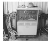
Miller Syncrowave 300 AC/DC Gas Tungsten Arc Welder w/Foot Control & Argon Atch. 200/230/460 Single Phase
