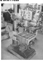
**Modigs Type RPM 28 BL Swing Arm Radial** Drill 1400 to 2800 RPM, Max Distance From Column to Center of Spindle 2' 3 3/8", Min. 9 1/4"
