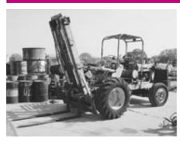
Windham Mdl. W-10 All Terrain Forklift, 4 Cyl. Diesel Engine, 10,000 Lb. Lift, 13' Two Stage Mast
