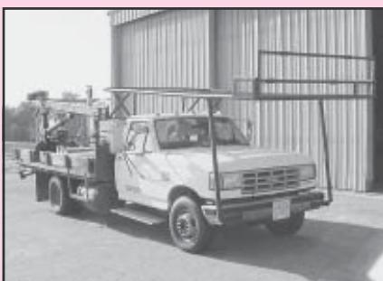
1990 Ford Super Duty Retrieval Truck, 7.3 L Diesel 5 Speed, Dual Tanks, AC, AM/FM, 96,000 Miles, 12' Flatbed, Hyd. Boom with Overcab Wing Rack
