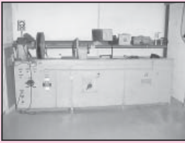
Sperry Magnaflux Machine, Mdl. BPM-120, 10' Bed, 220/440 3 Phase, 6000 Amp D.C. Output, 1200 Amp Continuous w/ DeMag
