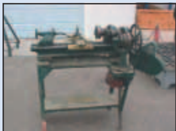
Southbend Lathe 36" Bed, 9" Swing, 3 Jaw Chuck
