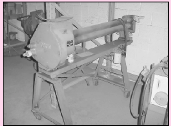
Pexto 416E Power Sheet Metal Roller, 48", 14-16 Ga. Soft Steel
