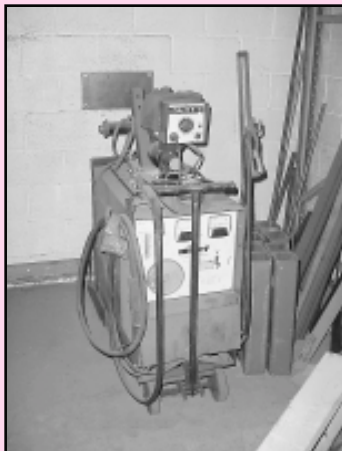
Miller Model CP-300 DC-Welding Source w/Miller Matic 10-E Wire Feed Attach.
