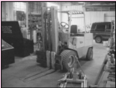
Yale GP080 8,000 Lb. Forklift, Gas, Pneumatic Tires, Two Stage, 12' Lift Big Joe Model 2018-R6 Electric Pallet Jack
