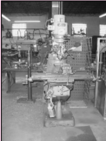
Enco Model 2VS Vertical Milling Machine, 2 H.P. Head, 500 to 4,200 RPM, 36" Table
