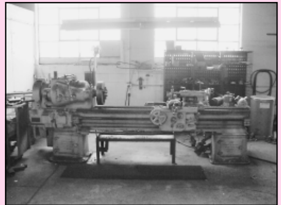
Boyd & Emmes Machine Tool Lathe, 18", 8' Bed, 1 1/2" Hollow Spindle, 3 & 4 Jaw Chuck, Steady Rest and Various Other Attach.
