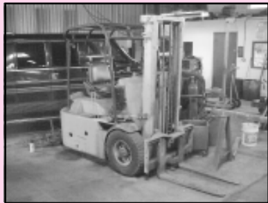
Hyster H-40 Spacesaver 3 Wheel Forklift, 4,000 Lb. Full Free Lift 10', Pneumatic Tires (2 Ea.) 4,000 Lb. Pallet Jacks
