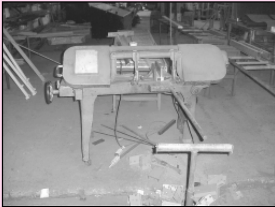
Kalamazoo Model 8166 Metal Cutoff Saw
