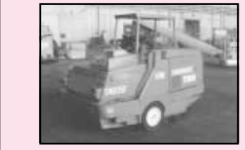
Tennant Model 95AA Drive Around Hangar Sweeper, 4 Cyl. Gas Engine with Hyd. Controlled Brooms
