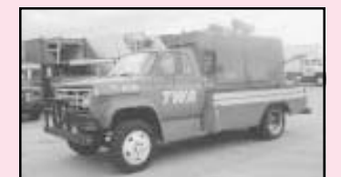
GMC Sierra 5000 Air Start Truck with Sprague Model JSS-DSP Compressor Unit, Caterpillar Diesel Engine (2 Ea.) GMC-6000 Air Start Trucks, Manual Trans., V-8 Engines with Stewart Stevenson Model TRAC-135 Compressor Units, Detroit Diesel Engines
