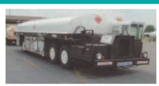
Dart 8,000 Gal. Low Profile Avgas Truck, Steel Tank with Fresh Epoxy Lining, Dual Pumps and Meters, (1) Single Point Hose, (1) Overwing Hose, Top and **Bottom Load, Cummins Diesel Engine**
