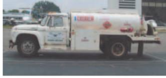
1966 Ford 1,200 Gal. Avgas Truck, Steel Epoxy Lined Tank, Single Pump, Meter and Reel, Top and Bottom Load, V-8 Engine, 4 Speed Trans.
