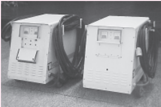
(2 Ea.) Trilectron LP28-400 Start Carts (Near New) Input 440 V 25-100 Amps 3ph 60 Hertz Output 28V 400-2000 Amps
