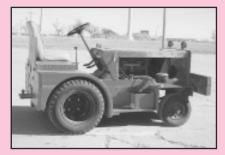
Minneapolis Moline 4,000 Lb. Aircraft Tug, 4 Speed, 6 Cyl. (2 Ea.) Hobart Jet Ex III Ground Power Units, 28 Volt, 750 Amp Continuous, 1500 Amp Peak, 6 Cyl. Ford Engine, (1) Unit has Voltage
