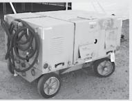
Liquidonies MdI AHT-64 Diesel Engine Driven Hyd. System Test Stand, Dual System, 20 G.P.M @ 3,000 PSI. Empire BBO Basket Blaster w/Filter
