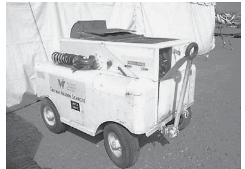
Airesearch Mdl AIAENC Air Start Cart w/Garret GTC 85-70A Turbine Engine
