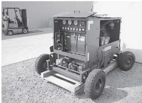
Automatic Military Air Start Cart Type MCII, 2 Cyl Diesel Engine, 15CFM at 4,000 PSI
