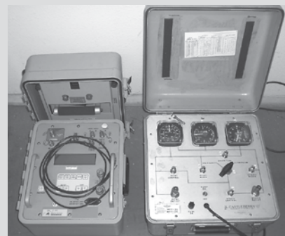
IFR-601 Digital Ramp Test Set IFR-401L Nav Ramp Test Set
