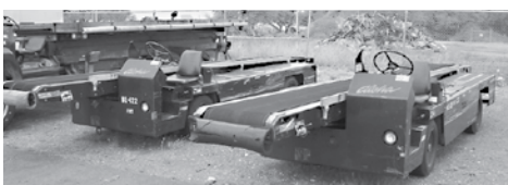
(2) Stewart Stevenson Mdl 660-11 Belt Loaders, 6 Cyl. Gas Engine, 2,000 LB, 24' Belt, Mfg in 2000 & 2002
