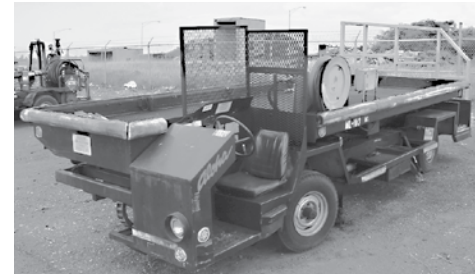
Wollard Mdl TML-704 Maintenance Scissor Lift Truck, Diesel Engine, 17' x 7' Bed, Lift Height 16', 2,000 LB Capacity
