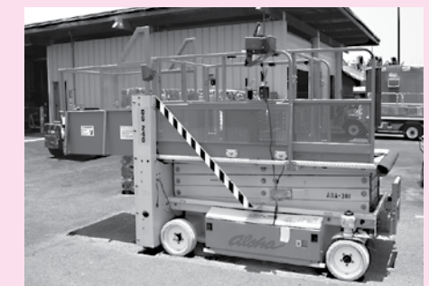
JLG Mdl. 2658E Wheel Chair Lift, Electric, 1,000 LB Capacity
