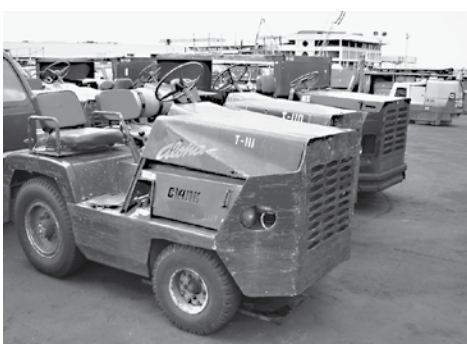
(11) Clark Mdl CT-30 Baggage Tugs, 3,000 LB D.B.P., 6 Cyl. Propane, Auto Trans. (2) Stewart Stevenson MA-50 Baggage Tugs, 5,000 LB D.B.P., 6 Cyl. Propane (2) United Baggage Tugs, 3,000 LB D.B.P., Auto Trans., Perkins Diesel Engine
