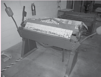
Tennsmith U48-12 Finger Brake, 48", 12-Gauge Capacity
