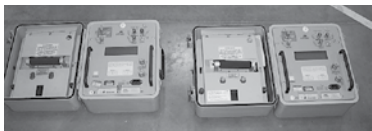
(5) IFR ATC-601-2 Transponder Ramp Test Sets for ATCRBS & Mode S XPDP's
