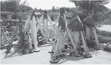
(2) Malabar Mdl 759A 50-Ton Tripod Aircraft Jacks, Air Over Hydraulic Malabar Mdl 718-A 20-Ton Nose Jack, Air Over Hydraulic
