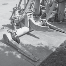
(2) Malabar Mdl 60P10 60-Ton Axle Jack, Air Over Hydraulic
