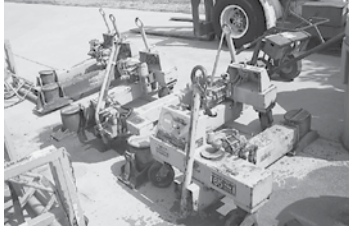
(2) Malabar Mdl 767A 60-Ton Tripod Aircraft Jacks, Air Over Hydraulic
