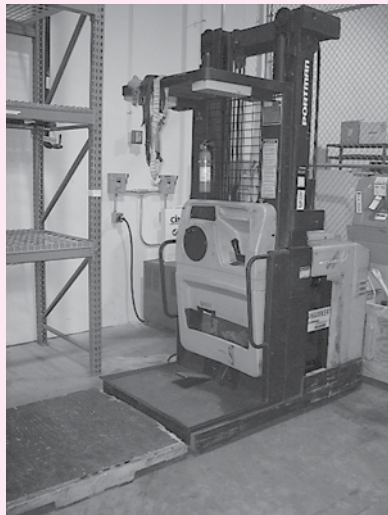
Hyster Mdl E45FR Electric Standup Forklift, 3,800 Lb, 18' Triple Stage Mast, Side Shift Forks, New Battery
