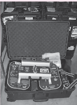
(5) DBI Sala Self-Contained Vacuum Anchor System (Personal Fall Protection Systems) w/Suction Cups & Nitrogen Bottles
