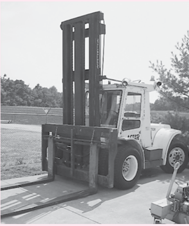
Hyster Mdl H200HS All Terrain Forklift, 13,400 Lb, Dual Stage Mast, 212 In. Diesel Engine, Side Shift Forks
