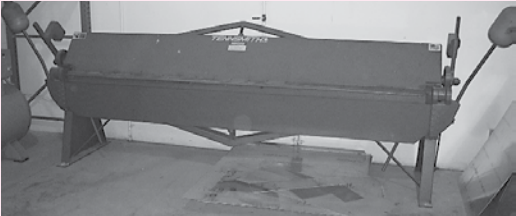
Tennsmith Mdl HB12116 Sheet Metal Brake, 10', 16-Gauge Capacity
