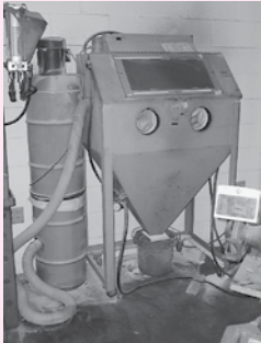
Dayton Mdl 3Z850 Bead Blast Cabinet w/Filter
