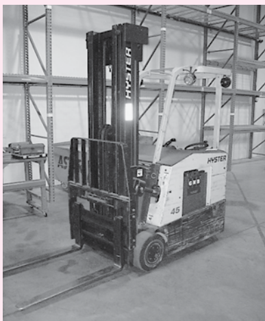
Hyster Mdl E45FR Electric Standup Forklift, 3,800 Lb, 18' Triple Stage Mast, Side Shift Forks, New Battery
