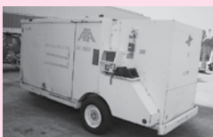
Stewart Stevenson Mdl TMAC-250 Air Start Cart w/Detroit Diesel Engine, 250 LBS Per Min @ 32 PSIG
