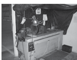
Magnaflux Type MAG II-60 Magnaflux Machine, AC/DC, 5,000 AMP, w/DeMag, 7' Bed
