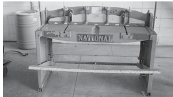
National Mdl 5216, 52" Sheet Metal Shear, Cap 16 Gauge Soft Steel
