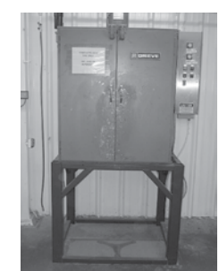
Grieve Mdl 333 Electric Oven, 400° F, 36" x 36" (Inside Measurement)
