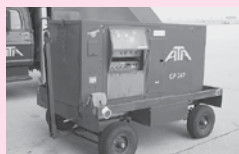
Stewart Stevenson Mdl TM-4900 Ground Power Unit, Detroit Diesel Eng, 90 KVA
