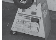
Universal Bead Blast Cabinet w/ Reclaimer & Filter System, 4' x 4' x 4'
