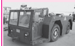
Stewart Stevenson Mdl GT50H Push Back Tractor, 60,000 LB, Caterpillar Diesel Engine
