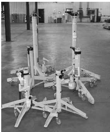
(2) Meyers 60" Tripod Jacks, 5-Ton Capacity (7) Meyers 25" Tripod Jacks, 8-Ton Capacity
