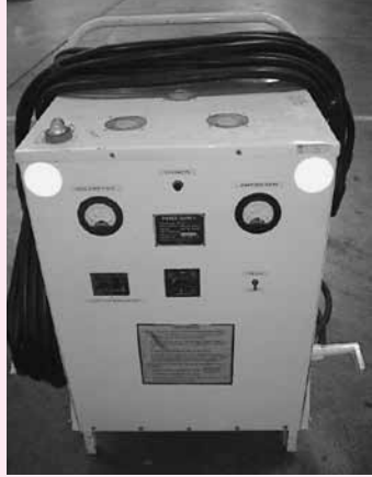
U.S. Power Supply Type B9, 400 Amps, 28V DC Output, 220, 60 Hz 3-Phase Input
