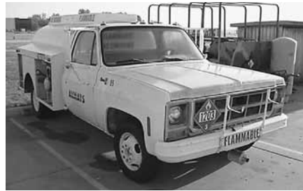
1980 GMC 3500 Avgas Fuel Truck, 750 Gallon Steel Tank, Single Over Wing Nozzle, 60 GPM, Top & Bottom Load
