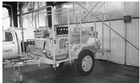
2007 Military Generator Trailer w/2ea. Onan Diesel Generators, 400 Hz/10 KW Each, New From Military, 2 Hrs. T.T.
