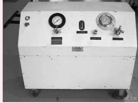
Jet Mac 5606 Hydraulic Mule P/N 1006-SA-3, 0-10 GPM, 3,000 PSI Arnolt Corp CPT-6A Cabin Pressurization Cart, 6-Cyl Packet Engine
