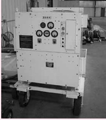
Triletron Frequency Converter Mdl 15SS400, Input 480V, 3-Phase Output 115-200V, 400 Hz, 15 KVA, 12 KW
