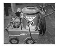
Hotsy MdI 550 B Heated Pressure Washer; 2.2 GPM; 1000 PSI; SgI Phase
