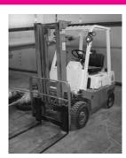
Nissan Mdl NF01: 3000 Lb Fork Lift: 12' Dual Stage Mast; Pneumatic Tires; Gas Eng
