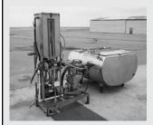
(3) Chemical Mixing & Transfer Pump Rigs; 1 is Portable Pace Transfer Pump w/5HP **Briggs Eng** (2) Electric Transfer Pumps
