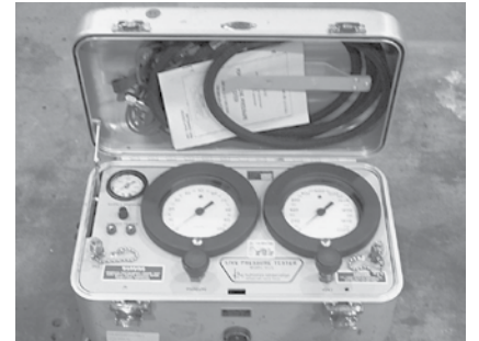
King Portable Live Pressure Test Set Mdl 3112 Tanma Digital Dual Power supply 35V-10A (8) Engine & Module Slings
