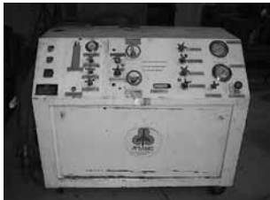
Jet Mac Mdl 1006-SA-4 Hydraulic Mule, Cap 0-10 GPM @ 3,000 PSI, Skydrol 500B or Equivalent Fuel
