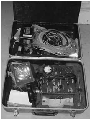
Chadwick Vibrex Track & Balance System w/Mdl 177M-6A Balancer & 135M Strobe
