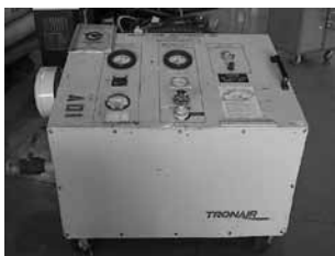
Tronair Mdl 15-7602-1000, 80 Cabin Pressurization Unit, Pressure Range 1-12 PSIG, Air Flow 0-240 ACFM
