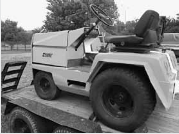
Clark Tug 4,000 Lb DBP, Ford Straight 6 Engine, Auto Single Speed Transmission
