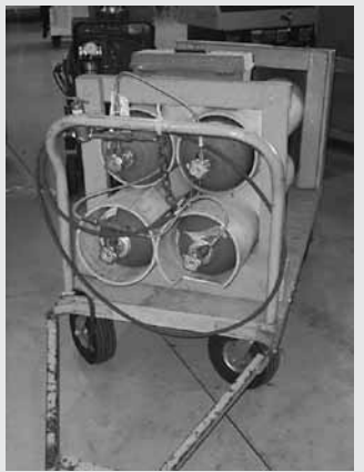
Tow Behind 4-Bottle Oxygen Cart w/ Gauges, Regulators & Bottles
