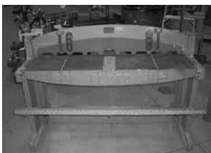
Pexto Mdl 152 Sheet Metal Shear, 52", 16 Gauge Gap
