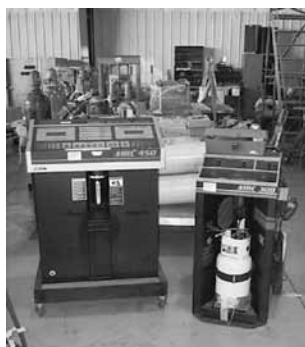
Sun Mdl MRC-450 Mobile Air Conditioning Recycling Center R-134A
