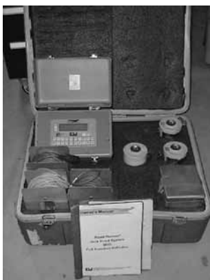
Evergreen Roadrunner Jack Point System Digital Aircraft Scale w/3ea 50,000 Lb Load Cells Evergreen Ramp & Pad Type Aircraft Scales w/Digital Readout Unit & (3) 0-2,500 Lb Pads
