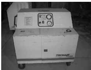
Tronair Mdl 05-7023-1100.81.7 Hydraulic Mule, Cap 0-10 GPM @ 3,000 PSI, 5606 Fluid
