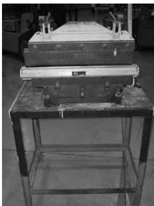
DiArco 25" Bench Top Press Brake, Hand Operated
