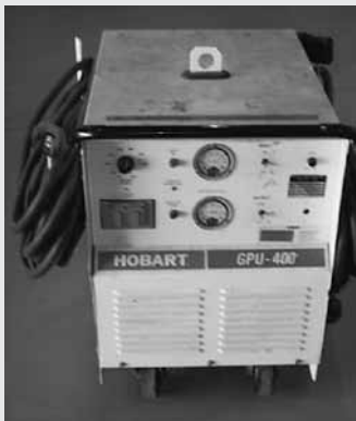
Hobart GPU-400 Mdl 6T28-400CL, 28.5 Volt, 400 Amp
