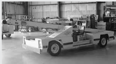
Cochran 660 Series Belt Loader, 2,000 Lb Cap., 24' Belt, Ford 6-Cyl Engine
