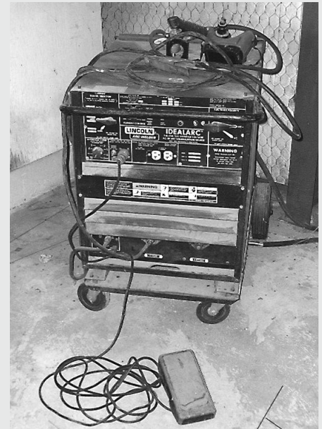
Lincoln Idealarc Tic 250 Variable Voltage AC/DC Arc Welding Power Source 208, 230/460 Volt, 1 Phase Input
