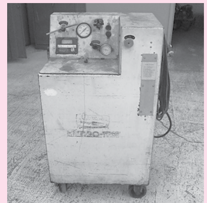
Cessna 3,000 LB Hydro Test Mule
