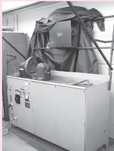
Magnaflex Type DR-543 Magnaflex Machine 6' Bed, AC Volts, 3000 Amps Max w/Black Lights
