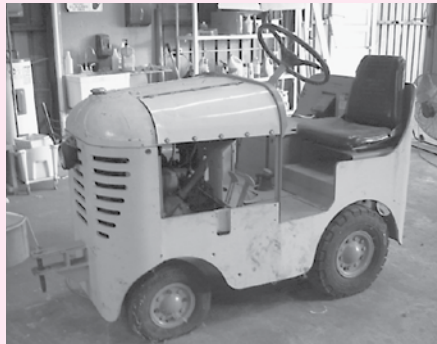
Clarkat Mdl. CK26F Aircraft Tug, 3 Speed, Flat Head 4 Cyl Engine, 2,000 lb DBP
