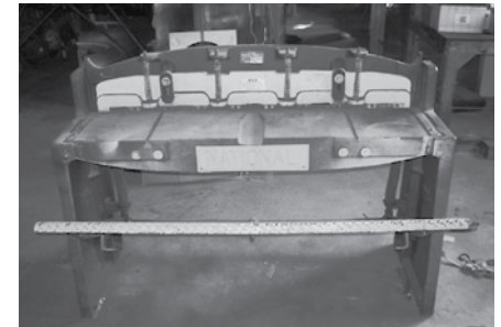
National Mdl. 5216 52" Sheet Metal Shear, 16 Gauge Mild Steel
