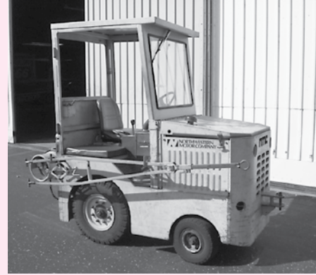
North Western Type LP30 Aircraft Tug, 3 Cyl Propane Engine, 3,000 Lb DBP
