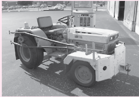
Kubota Mdl. B9200HST-D Tug Tractor, 4 Cyl Diesel, Hydrostatic Shift, 4 Wheel Drive Rhino Mdl. SE5 Brush Hog Mower, 3 Point Rhino Mdl. RF60 Flail Mower, 4 Ft Wide
