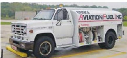
GMC 6000 Fuel Truck; 2500 Gal Aluminum Tank (Used for Diesel Fuel); 4 Compartment; Top & Bottom Load; Dual Reels; Single Meter; V-8 Engine; 5 Spd Manual Trans
