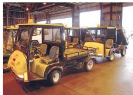
(2) Toro Workman 3200 Utility Vehicles; Liquid Cooled Daihatsu; 3 Cyl Gas Engines; 3 Spd Trans w/Lift Beds
