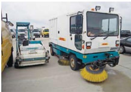
Tennant 830 Ramp Sweeper; Diesel Engine; 20,000 Lb
