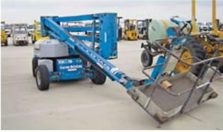
Genie Mdl Z-45/22 Manlift; Platform H 45'; 500 Cap; Propane
