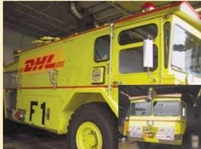
'72 Walter CBD-3000 Airport Fire Truck; (2) Detroit 318 Diesel Engines; Allison Trans; Continuous All Wheel Drive; 3,000 Gal. Water Tank; Foam Tank total of 180 Gal. of 3% A.F.F.F.; (2) Single Stage Hole Pumps; 1,000 G.P.M.; Top Turret Hakrom Pump (Spray up to 300 Ft.); Bottom Turret Santa Rosa Pump (Spray up to 125 Ft.); This Truck can Pump & Drive at the same time.
