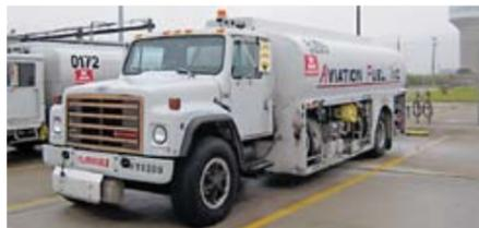
GMC 700 Fuel Truck; 5 Spd Trans; V-8 Engine; 2000 Gal; 5 Compartment Tank; 1000 Gal Diesel; 1000 Gal Gas; Dual Pump & Reels; Top & Bottom Load; Progress Industries Tank
