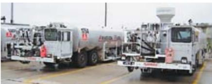
(2) Dart Mdl 150RFT & 100FTDR 10,000 Gal Low Profile Jet A Fuel Trucks; Aluminum Tanks; 653 Detroit Diesel Engines; Allison Trans; Top & Bottom Load; De-fuel Capable; Dual Single Point Under Wing Nozzles in Front; (1) Single Point Nozzle on Side. Filter Elements Current through '09; Voyager Backup; Cameras for Rear & Sides
