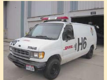
'00 Ford E-350 Panel Van; 4.2 L; V-6; Setup for Hazmat Response
