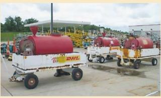
(3) Par Kan Mdl. FSC-300 Fuel Carts w/250 Gal Tanks, Hand Pumps
