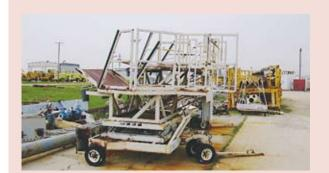
(Approx. 20) Build by Southworth Mdl LS4-48W, 4,000 Lb. Cap., Adjustable Height w/Electric Motor, Some have 30' Conveyors Included that have Onan 7.5 KW Generators & Diesel Engines. Used to Load C-Containers in the Belly of 767's.
