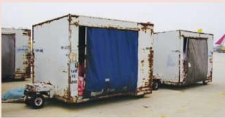
(60+) Belly Freight Wagons built by Clyde Mdl F2498 & P&G Fabricating Units. Measure 144" L x 92" W x 96" Tall and Enclosed on 3-Sides & Open on 1 Side.
