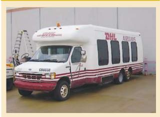
Ford E-350 Crew Shuttle Bus, Ford 7.3 Liter Diesel Engine, Auto Trans w/Overdrive, Dual Air, Hoekstra Body.
