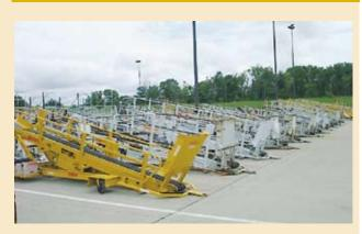
(Approx. 60) Conveyors, Various Lengths, All Have Adjustable Heights. Some were Mfg. by Scott Randell Conveyor Systems, Some by WHM Conveyor Systems, All have Onan or Lister Petter 7.5 KW or Bigger Generators w/ Diesel Engines, Belt Lengths Include: 50' for DC-8's, 40' for 767 Bellies, 30' for DC-9's, and 18' for Truck Loading, Various Weight Capacities, for Loading C-Containers.
