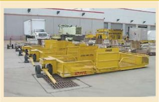
(18) C-Container/Wheel & Brake Carts includes a Combination of Clyde Mdl. F2129 & P&G Mdl 96014. Carts Measure 6'4" W x 15'3" Long and have Flip Down Ramps on Both Sides. These were built to haul (5ea) C-Containers at a time, could also be used as (and are identical to) other Wheel & Brake Carts.
