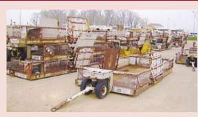
(65+) C-Container/Wheel & Brake Carts. Combination of Clyde Mdl F2129 & P&G Mdl 96014 Carts. Measure 6'4" W x 15' 3-3/4" L and Have Flip Down Ramps on Both Sides. These were built to haul (5ea) C-Containers at a time. Could also be used as/and are identical to other Wheel & Brake Carts.
