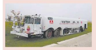
Dart 10,000 Gal. Low Profile Jet A Fuel Truck, (2) Under Wing Single Point Nozzles, (1) Single Point Side Nozzle, Top & Bottom Load, Fuel & De-Fuel Capable, Wilco 10,000 Gal Steel Coated Tank, Caterpillar Diesel Engine (Needs Some Work).
