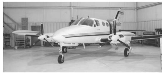
"1976" Cessna 414, N-456ST, S/N 414-0810. Total Airframe Time: 7,067 Hrs. Engines: Continental TS10-520-N's, Left Engine: 1,204 Hrs. S.M.O.H. by G&N, Right Engine: 1,241 Hrs. S.M.O.H. by G&N, Props: McCauley 3 Bladed (Ram STC), Left Prop: 602 Hrs. S.O.H., Right Prop: 744 Hrs. S.O.H.
