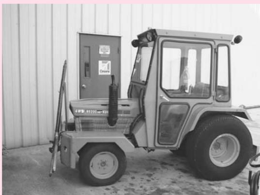
Kubota Mdl. B9200 Tug Tractor 4 Wheel Drive, 4 Cyl. Diesel, Hydro-Static Drive
