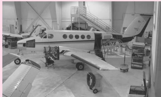
1980 Beech King Air 200, N-641TS, S/N BB-641. Airframe Total Time: 10,444 Hrs., **Note:** Nose gear had collapsed on the aircraft causing damage to nose & rear fuselage. The nose repairs are nearly complete. Rear fuselage repairs are being made. Engines: P&W PT6A-41, Both engines were damaged and are totally disassembled and will be sold that way. Props: Both props are damaged.
