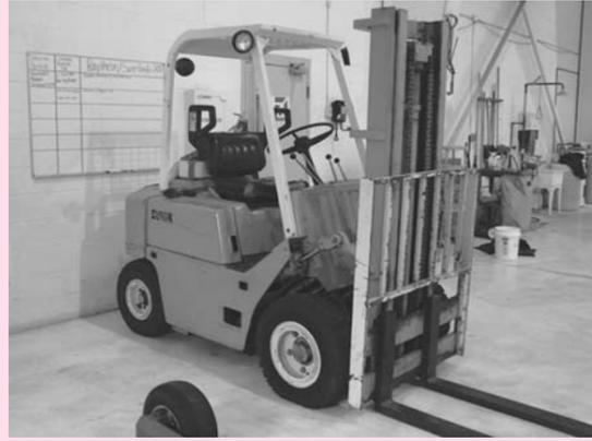
Clark Mdl. C500Y40 Fork Lift 4000 Lb. 10' Dual Stage Mast, Pneumatic Tires, Gas
