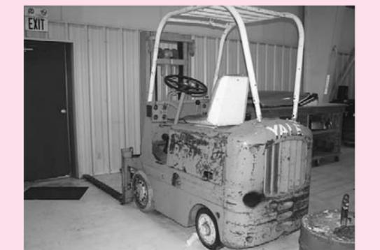
Yales Mdl. KG51AT-40U Fork Lift, 5000 Lb., 10' Dual Stage Mast, Hard Rubber, Gas
