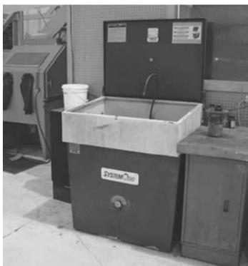
Mansur Mdl. 500 System One Heated Parts Washer w/ Recycle & Sludge Removal System
