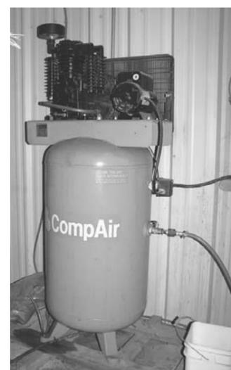
Compair Mdl. K-3-5N8V13 Vert. Air Compressor, 5 hp, Dual Stage
