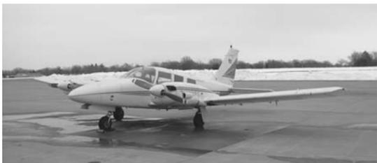
"73" Piper PA-34-200 Seneca I, N-16558, S/N 34-7350159. Total Time Airframe: 3,778 Hrs., Engines: IO-360-CIE6, Left Engine: 3 Hrs. S.M.O.H. by Signiture, Right Engine: 1,876 Hrs. S.M.O.H., Hartzell Props: Left Prop: 3 Hrs. S.O.H., Right Prop: 2297 S.O.H.
