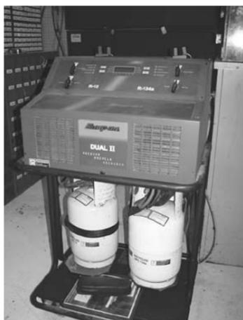
Snap On Dual II Air Conditioning Recover, Recycle, Recharging Sys. for R-12 & R-134A
