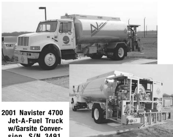
2001 Navistar 4700 Jet-A-Fuel Truck w/Garsite Conversion, S/N 3491, Done 09/01, 581 Miles on Truck, 3 Spd. Automatic Trans., Int'l. T-44E Diesel Eng., 3000 Gal. Stainless Steel Tank, Load Rate 300 GPM @3.0 PSIG Unload Rate 350 GPM, Bottom & Top Load, Single & Over Wing Nozzles & Reels, Facet Filter Sys. Filters Changed 08/06.
