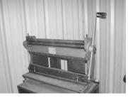
Central Machinery Mdl. T-2079 3 in 1 Sheet Metal Machine, Brake, Shear, Roller 30", 16 Ga. Cap
