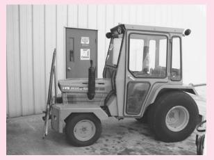
Kubota Mdl. B9200 Tug Tractor 4 Wheel Dirve, 4 Cyl. **Diesel, Hydro-Static Drive**
