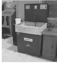
Mansur Mdl. 500 System One Heated Parts Washer w/ Recycle & Sludge Removal System
