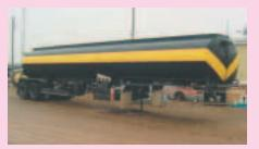
1971 Fruehauf 8.500 Gal. Nurse Rig Aluminum Four Compartment Tank Compartment #1 - 3,000 Gal. Jet A Fuel, Compartment #2 - 1,500 Gal. Jet A Fuel, Compartment #3 - 1,500 Gal. and Compartment #4 - 3,000 Gal. Water and Chemical Storage, Hydraulic Flow Control Pumps, Meters for Fuel and Chemical, 3" Chemical Pump, 2" Fuel Pumps
