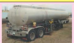
1969 Wilco 8,000 Gal. Nurse Rig **Aluminum Five Compartment Tank** Compartment #1 - 2,400 Gal. Jet A Fuel, Compartment #2 - 1,000 Gal. Jet A Fuel, Compartment #3 - 1,000 Gal. and Compartment #4 - 1,400 Gal. (Water and Chemical Storage), Compartment #5 - 2,000 Gal. Mixing Compartment. All Chemical and Fuel Pumps are Hydraulic Controlled, Fuel and Chemical Meters. Fuel is Top and Bottom Load
