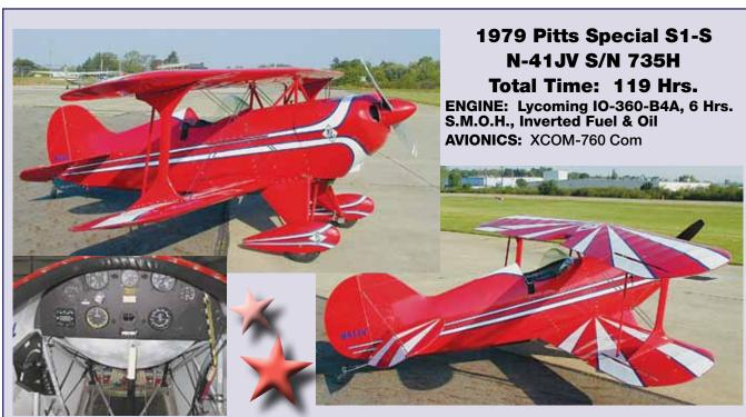
Aircraft was Disassembled, Refinished & Recovered in 1997. Fuselage, Wings & Control Surfaces were Inspected and Recovered with Superflite Process w/102 Fabric, SF-250 Primer & Superflite Finish. Reassembled with all New Hardware.
