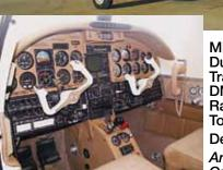
Microline, Dual Collins VHF-251 Coms, Dual Collins VIR-351 Navs, Collins TDR-950 Transponder, Collins ADF-350, King KN-62 DME, King KI-226 RMI, Bendix RDR-150 Radar, King KFC-200 Autopilot, Shadin Fuel Totalizer, Sigtronics Intercom.
