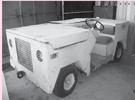
Consolidated Diesel Electric Model NC-8A Mobile Electric Power Plant, Has Detroit Diesel Engine, DC-Output 28V, 500 Amp Continuous DC-Output 28V, 750 Amp Starting Duty, AC-Output 3 PH, 120/208 V, 167 Amps, 400 Cycle, 60KVA
