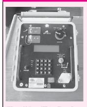
IFF-701TI IFR MdI Ramp Transponder Test Set, S/N 701007674, Still in Calibration
