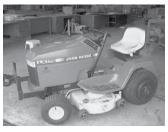
John Deere LX176 Lawn Mower 38" Deck, 19 HP Briggs, Hydrostat Drive
