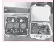
AIS ADT-3543E Pitot Static Test Set w/SA3Y-P Test Adapter Set
