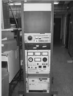
Elgar Programmable AC Power Supply Mdl 55974-3599948-1 & Unitron Mdl CR074-3A Power Frequency Converter, 50/60 Hz, 30 (WYE) to 400 Hz, 30 WYE
