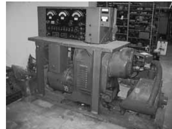
United Type A-1 Aircraft Generator Test Stand (Vari-Drive), 25-HP Motor, 12,000 RPM, Single Head w/Cooling Fan, 600 Amp Load Bank
