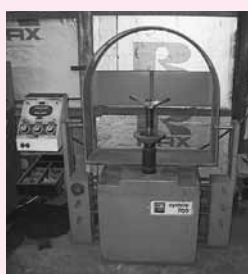
Hunter System 700 Computer Wheel Balancer, 500 RPM Balancing Speed
