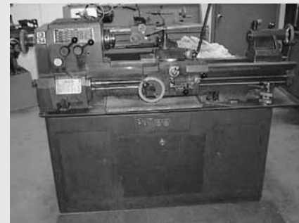
Standard-Modern Mdl 1334 Lathe, 13" Swing over Bed, 48" Bed, 34" Between Centers, 36-1,800 RPM Spindle Speed
