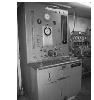
Air Associates Inc Mdl TE872 Hydraulic Pump Test stand, Skydrol, Up to 5,000 PSI, 7-10 GPM
