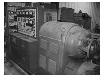
United Type A-2 Generator Test Stand, Vari-Drive, 50-HP Motor, Dual Head 2,350-9,000 RPM Low Side, 3,000-11,500 RPM High Side w/550 Amp Load Bank
