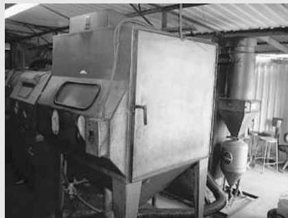
Universal Pressure Blast Cabinet w/Dust Collector, 48" D x 48" W x 48" T Cabinet Size, w/Door on each side
