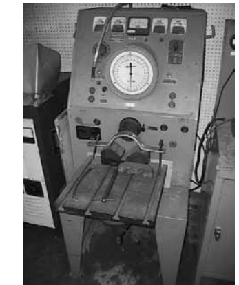
Potter-Rayfield Inc Mdl DM-15(AC-DC) Starter Motor Torque Tester, Rated Capacity 15 Ft/Lb Torque, 4,000 RPM Speed, 50 Amp
