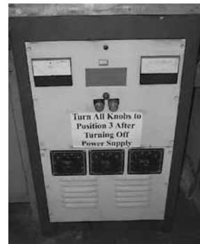
Clinton DC Power Supply Mdl S1012H0-2, AC Input: 230-Volt, 42-Amp, 60 Cyl.; DC Output: 6-12-Volt, 1,000 Amp, 12 KW
