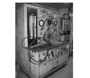
Sprague Mdl S529 Hydraulic Test Stand, 5606 Fluid, Up to 3,000 PSI, 6,000 RPM
