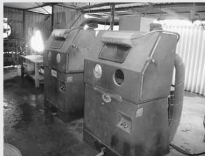
(2) Zero Mdl BNP-55 Bead Blast Cabinets w/ Reclaimers, 24" D x 42" W x 30" T Cabinet Size
