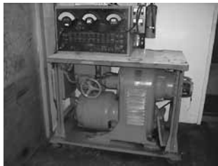
US Vari Drive Bench, 15-HP, 300 Amp Load Bank, Dual Head 2,400-12,000 RPM High Side, 1,100-5,500 RPM Low Side
