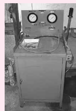
Brake Pressure Test Bench 0-160 PSI Low Pressure & 0-6,000 PSI High Pressure Parker Mdl DA-200 Contour Probe Shop Built Wheel Bead Brake w/Variou Size Rings
