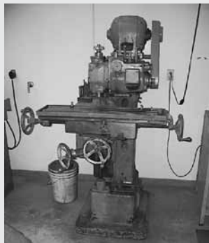
Van Norman No. 12 Horizontal Milling Machine, 37" x 9" 3-Slot Table, Head Spindle Speeds 70-1,465 RPM
