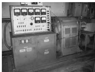
United Type A-2 Aircraft Generator Test Stand, Dual Head 2,350 RPM-9,000 RPM Low Side, 3,000-11,600 RPM High Side, 60-HP Motor, 500 Amp Load Bank
