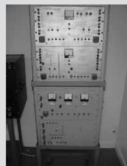
Lear Siegler DC Voltage Regulator Test Stand for 51509-001, -002, -006 Voltage Regulators & Lear Siegler DC Generator Control Unit Test Panel for 51530-006, -007 & -008 GCU's
