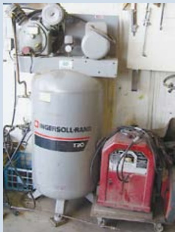
Ingersoll Rand 242-5N Vertical Air Compressor; 5 HP; Single Phase Motor; Dual Stage; 80 Gal Tank
