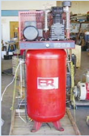
Big Red Mdl BRA 618V Vertical Air Compressor; 6 HP; Single Phase; Dual Stage; 80 Gal Tank
