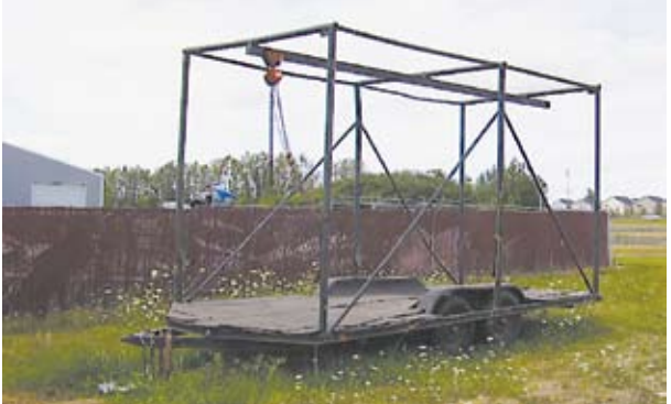
19' Aircraft Retrieval Trailer; Dual Axle; Overhead Chain Hoist & Trolley
