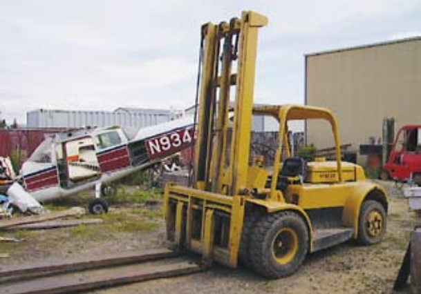
Hyster Mdl H120G Fork Lift; 11,000 Lb Cap; Diesel; 20' Dual Stage Mast; Side Shift Forks; Dual Front Tires
