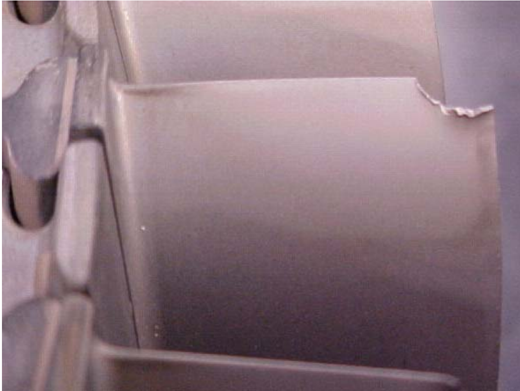
4 TH STAGE LPC BLADE NICKED ON LEADING EDGE
