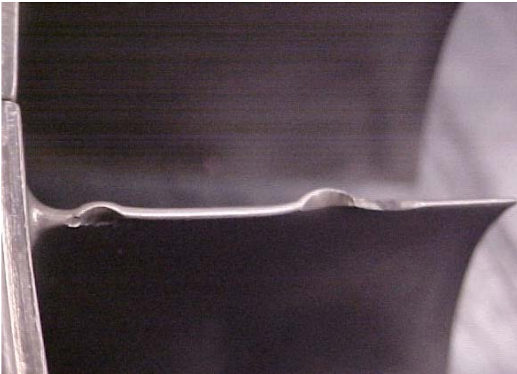
3 RD STAGE LPC STATOR VANE NICKED ON TRAILING EDGE
