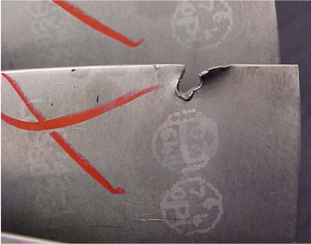
2 ND STAGE LPC BLADE NICKED ON LEADING EDGE
