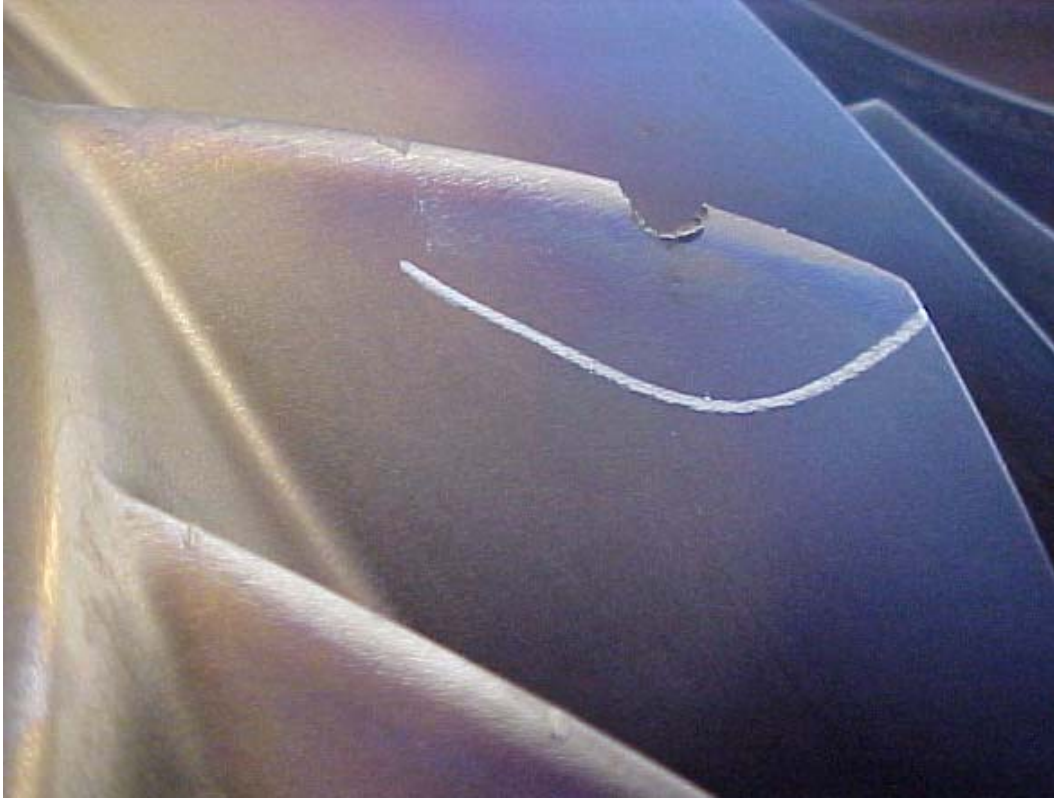
HPC IMPELLER VANE NICKED ON LEADING EDGE
