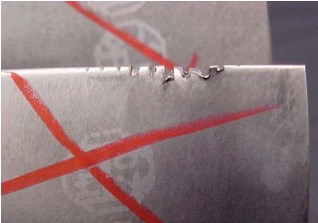
2 ND STAGE LPC BLADE NICKED ON LEADING EDGE
