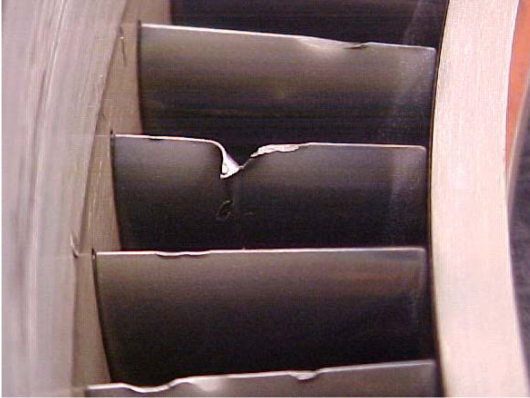
4 TH STAGE LPC STATOR VANES NICKED ON LEADING EDGE
