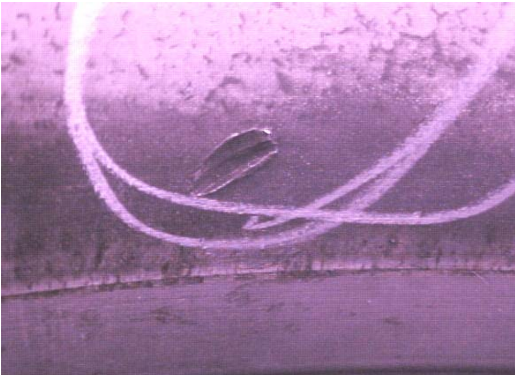
HPC IMPELLER SHROUD NICKED ON INNER SURFACE
