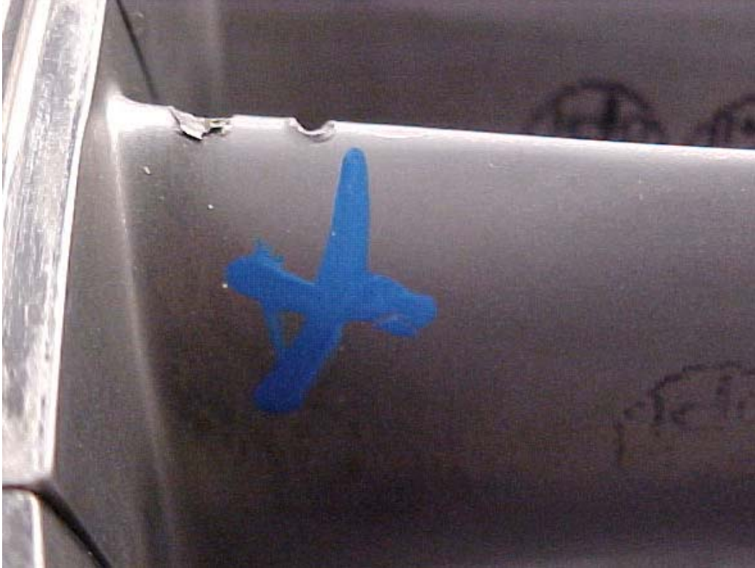
1 ST STAGE LPC STATOR VANE NICKED ON LEADING EDGE
