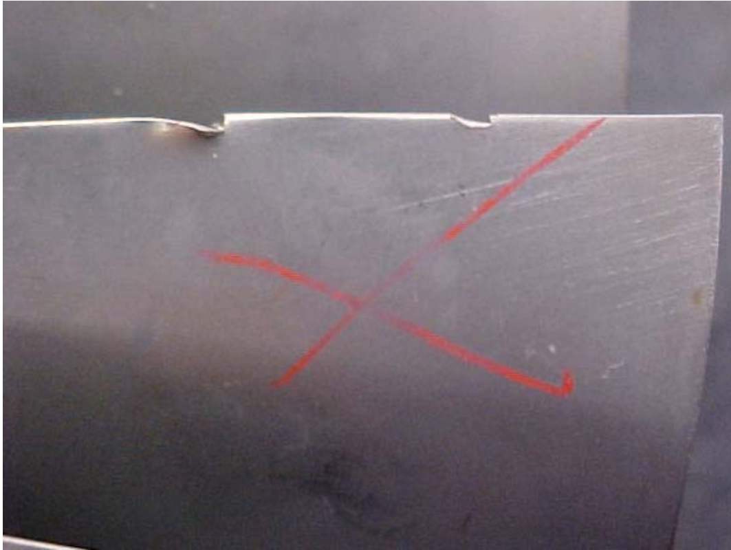
1 ST STAGE LPC BLADE NICKED ON LEADING EDGE
