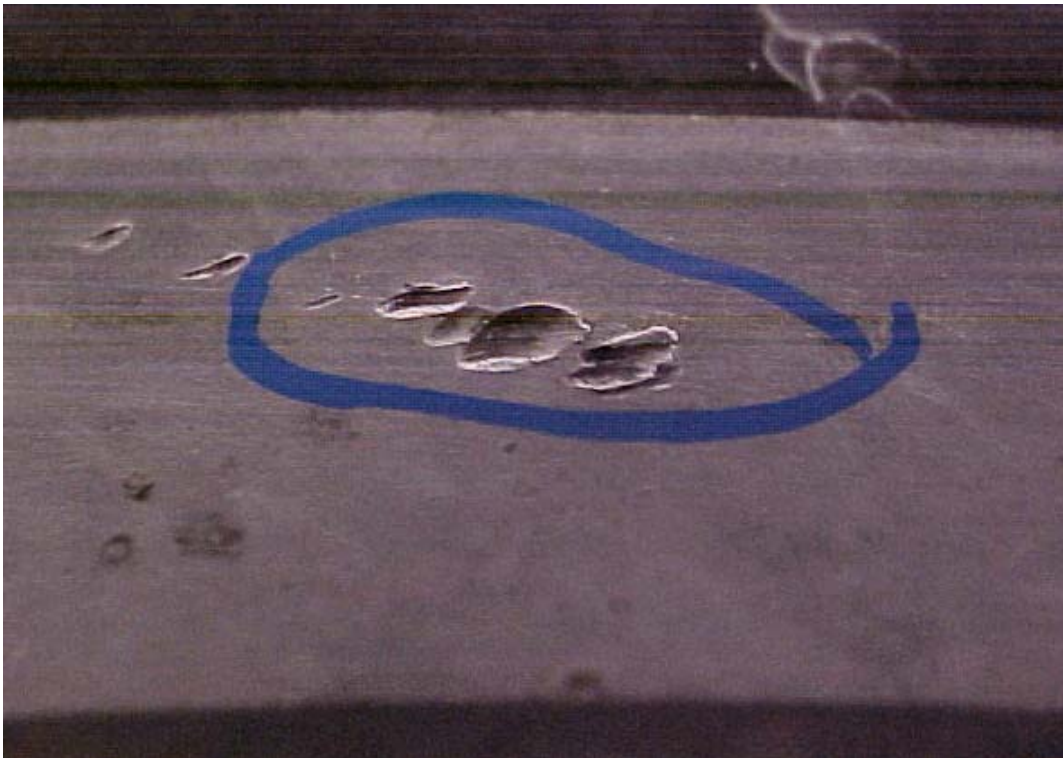
3 RD STAGE LPC STATIONARY SHROUD NICKED ON INNER SURFACE
