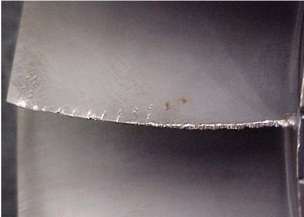
1 ST STAGE LPC BLADE NICKED ON TRAILING EDGE
