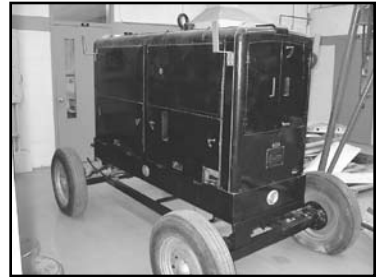
(2 Ea.) Hobart GPU Start Cart P/N 2361 30KW, 28V DC, 8 Cyl. Gas Chrysler Industrial Hemi Engine 400,000 BTU Portable Heater Mdl. BT-400-30
