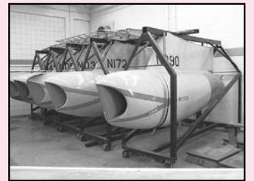
(5 Ea.) Westinghouse J34-36A Engines in P2-V Neptune Nacelles on Carts (Most w/Hard Card Logs)
