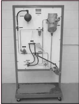
Avotek Mdl. H37 Hyd. System Training Board, Has Cylinders, Hand Pump and Accumulator (4 Ea.) Nav. and Landing Light Training Boards (All Have Landing Lights and Motors)
