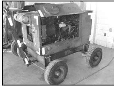
Davey Mdl. MC1A Airstart Cart 15 CFM at 3,500 PSI, 4 Cyl. Wisconsin Gas Engine Herman Nelson Mdl. GT 3090D Portable Heater Cart
