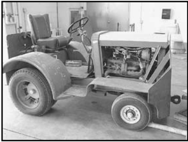
Clark CT40 Tug 4,000 Lb. D.B.P., 6 Cyl. Flat Head, Gas, Manual Trans. Hobart Mdl. 488 25 H.P. 600 Amp 28V Generator Cart
