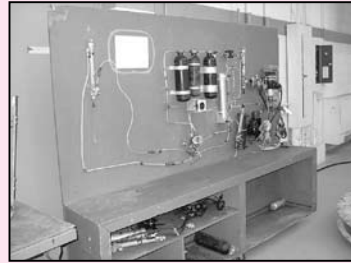
(3 Ea.) Actuator and Hyd. Training Aid Boards w/Electric Motors, Multiple Actuators and Accumulators
