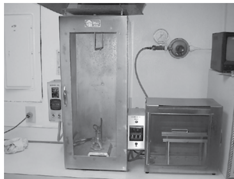
Seat Cushion Burn Testing Station, w/Control Panel, Video Monitoring / Recording
