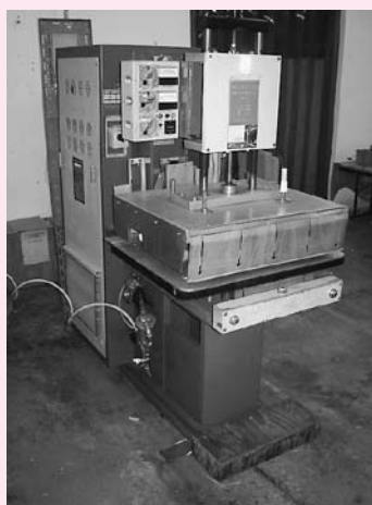
(3) Hall Dielectric Machinery Co. Mdl. FS-4-6A Radio Frequency Heat Sealing Machine, 6 kw RF Power Output, Freq. 27.12 Mhz, Bed Plate 33" x 27", Heated Platen 24" x 20", Throat Size 15", 7" Stroke, 1300 Lbs Down Pressure at 100 PSI.
