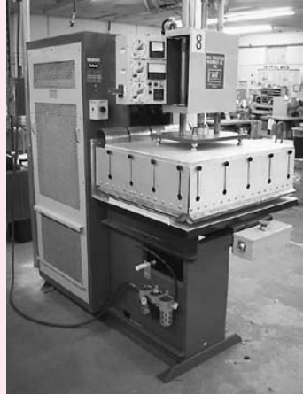
Hall Dielectric Machinery Co. Mdl. FS-10A Radio Frequency Heat Sealing Machine, S/N 1255, 10 kw RF Power Output, Freq. 27.12 Mhz, Bed Plate 33" x 27", Heated Platen 24" x 20", Throat Size 15 1/2", 8" Stroke, 2827 Lbs Down Pressure at 100 PSI
