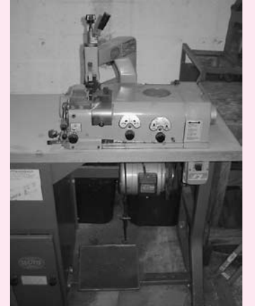
Sagitta Mdl. SC75B Skiving Machine Eastman Long Handle Pull Cutters
