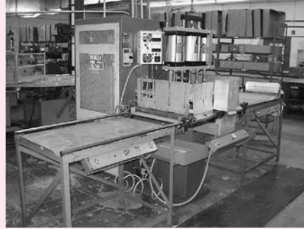
(2) Hall Dielectric Machinery Co. Mdl. FS-15A Radio Frequency Heat Sealing Machine, 15 kw RF Power Output, Freq. 27.12 Mhz, Bed Plate 33" x 27", Heated Platen 24" x 20", Throat Size 16 1/2", 8" Stroke, 2827 Lbs Down Pressure at 100 PSI, Manual Side to Side Slide Tray Shuttle
