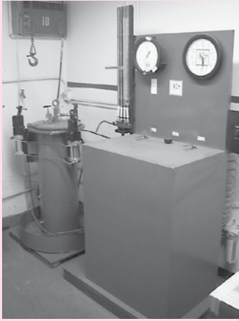
Hydro-Test Products Mdl. 500-08-14P Hydro Static "Water Jacket" Cylinder Test System, S/N 7262, Manually Operated, High Pressure Test Range 2,500 PSI – 10,000 PSI, 14" x 40" Water Jacket
