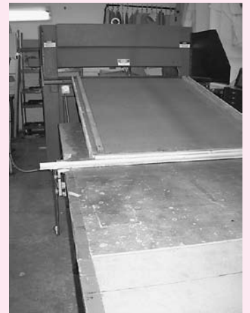
(2) Hall Dielectric Machinery Co. Mdl. FS-15A Radio Frequency Heat Sealing Machine, 15 kw RF Power Output, Freq. 27.12 Mhz, Bed Plate 33" x 27", Heated Platen 24" x 20", Throat Size 16 1/2", 8" Stroke, 2827 Lbs Down Pressure at 100 PSI, Manual Side to Side Slide Tray Shuttle
