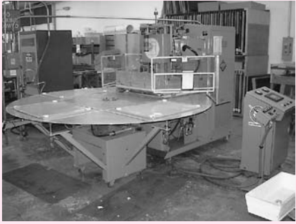
Cosmos/Kabar Mdl DH15,000 Radio Frequency Heat Sealing Machine, w/ 4 Station Rotating Turntable Camco Mdl. 902RDM4H32-330, S/N 00213064
