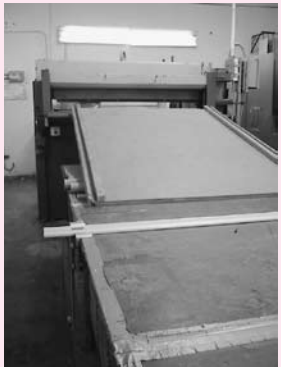
Hall Dielectric Machinery Co. Mdl. FS-10A Radio Frequency Heat Sealing Machine, S/N 1255, 10 kw RF Power Output, Freq. 27.12 Mhz, Bed Plate 33" x 27", Heated Platen 24" x 20", Throat Size 15 1/2", 8" Stroke, 2827 Lbs Down Pressure at 100 PSI
