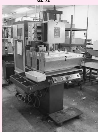
(3) Hall Dielectric Machinery Co. Mdl. FS-4-6A Radio Frequency Heat Sealing Machine, 6 kw RF Power Output, Freq. 27.12 Mhz, Bed Plate 33" x 27", Heated Platen 24" x 20", Throat Size 15", 7" Stroke, 1300 Lbs Down Pressure at 100 PSI.
