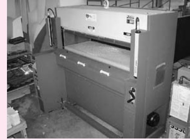
ATOM Series S3 Mdl. S325 Full Head Beam Cutting Press, S/N 10017951-1, w/ Rear Table, Working Width 1600 mm, Working Depth 600 mm, Max Pressure 25 Ton, Daylight Distance Between Plates 400 mm, Maximum Stroke 350 mm, Cutting Speed 65 mm Per Second, w/Sick Mdl. C4000 Photoelectric Safety Barrier Beam, Manufactured in 03, Installed in Plant 07, Was Factory Demonstrator
