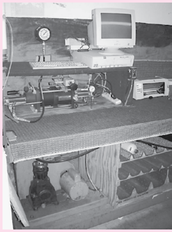
CO 2 and Nitrogen Cylinder Charging Station, w/ Haskel Mdl AGT-36/62 Pneumatic Gas Booster and Hydro-Test Products Mdl. SC-5 Transfer Unit
