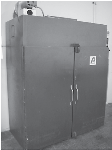
Precision Quincy Mdl 40D-350 Oven, S/N 27908, Mfd. 1985, 350° Fahrenheit Oven Temp, 2 Heater Banks, MEK & Tolvlo Solvents Used ½ Pint Per Hour, Purging Interval 4 Minutes
