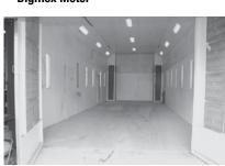
Viking Spray Booth; 40'L x 16'W x 15'H Rear Vent Bell 206 Fuselage Rebuild Jig (Not Factory Approved) ½" Stencil Cutting Machine
