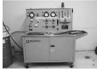
Starline SL-1200-15B-17 Skydrol Hydraulic Actuator Test Bench, Flow Rate 0-15 GPM, Adjustable Pressure 300-3500 PSI w/Hand Pump for up to 6,000 PSI Static Test Starline SL-1200-15B-17 5606 Hydraulic Actuator Test Bench, Flow Rate 0-15 GPM, Adjustable Press 300-3500 PSI
