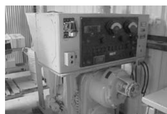
Shop Built Engine Driven Hydraulic Pump Test Stand 5,000 PSI
