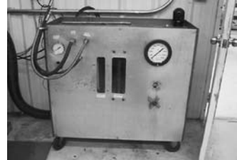
Shop Built Engine Driven Hydraulic Pump Test Stand 5,000 PSI
