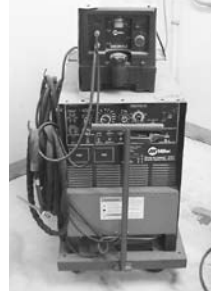
Miller Synchronwave 250 cc AC/DC Welding Power Source Tig Gun, Miller Cool Mate 3 Water Cooler, Foot Control Armature Cutter
