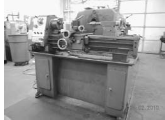
Enco Mdl 110-2072 Gap Bed Lathe S/N 886795, Mfg 1988, Metal Lathe, 10" Swing, 48" Bed, 1.5" Howell Spindle
