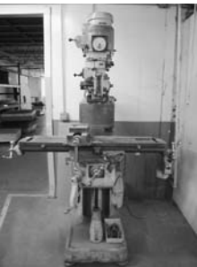
Bridgeport Series I Vertical Milling Machine, 1-1/2 HP Motor, 60-4200 RPM Spindle Speed, 9" x 42" 3-Slot Spacer, Auto Feed Table, 7" Riser Block
