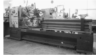
Crown Engine Lathe Mdl 4/200B, S/N C40120, Mfg 1981, 24" Swing, 3" Howell Spindle w/Tapper Attachment
