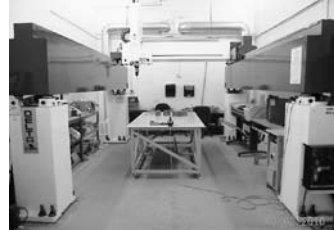
Delta DEA Mdl 3406 Gantry Type CMM, Measuring Envelope 128" x 72" x 54" (XYZ) PC-DMIS Software (2) Shop Built Submersible Fuel Pump Test Benches
