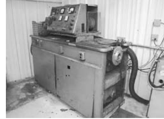
Generator Test Stand w/Sun Electric Mdl A-3 Veri Drive, w/Load Bank, 400/500 Amp, 25 HP Motor Drive RPM 2,000/Min, 11,000 Max
