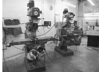
Lagun Republic FTV-1 Vertical Milling Machine, 3 HP, 50-3900 RPM, 42" x 9" 3-Slot Table, Auto Table Feed, Newall C80 Digital Readout X/Y Lagun Republic FTV-2 Vertical Milling Machine, 3 HP, 50" x 10" 3-Slot Table, 140-4200 RPM, Auto Feed Table & Knee Auto Height Adjustment, Topaz Digital Readout X/Y
