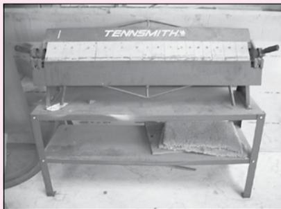
Tennsmith Mdl. U48 48" Finger Brake
