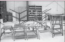
(4) 2-3' Maintenance Stands 5 & 6' Maintenance Stands (3) 4' Maintenance Stands Several Aircraft Jumper Cables **Misc. Bottle Jacks**
