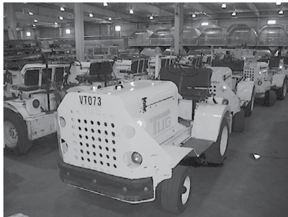
(7) Tug Mdl MA50-1 Baggage Tugs, 5,000 LB DBP, 6-Cyl Gas, Auto Trans
