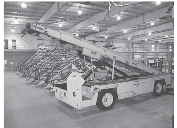
1994 S&S Tug Mdl 660-11 Belt Loader, 2,000 Lb Capacity, 6-Cyl Gas Engine, Wide Body Capable
