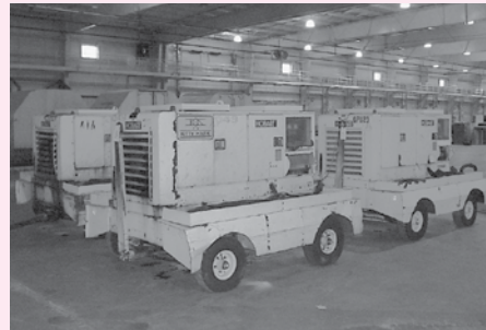
(4) Hobart Mdl 60-G20P GPU's, 60 KVA, Detroit Diesel Engines
