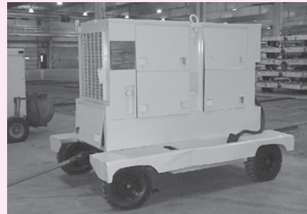
Kurtz & Root Mdl MEP115A GPU, 60 KW, 400 HZ, Allison Diesel Engine
