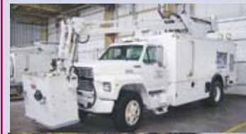
(2) 1995 FMC Commander 15 Universal Main Deck Loaders w/Wide Kit, Narrow & Wide Body Capable, w/Can Rotating Deck, Perkin 4 Cyl Diesel
