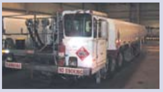
DART 10,000 Gal Low Profile Jet A Truck, 1 Sided Single Point Nozzle, 2 Under Wing Single Point Nozzles, Bottom & Top Load, Fuel/Defuel Capable, Facet Filter System, Detroit Diesel Engine, Brown Stainless Steel Tank
