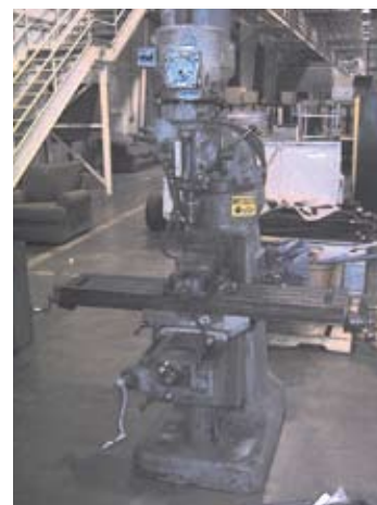
Bridgeport Mdl 108915 Vertical Milling Machine, 1 1/2 HP Motor, 9"x48" 3 Slot Table, 60-4200 RPM
