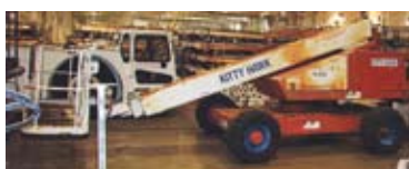
Snorkel Man Lift Mdl TB-42PR, Rebuilt, 4 Cyl, Wisconsin Engine 500 lb Cap Basket, Platform Height 42'
