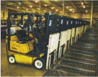
(34) Yale Mdl GLC030AFNUAV078 Forklifts, 3000 lb, Propane, Hard Rubber Tires, Dual Stage, 10 1/2 Mast, 5' Forks
