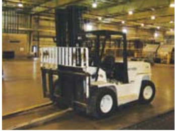
Hyster Mdl H155XL Forklift, 15,000 lb, Pneumatic Tires, Dual Front, Perkins Diesel, Triple Stage, 27' Mast
