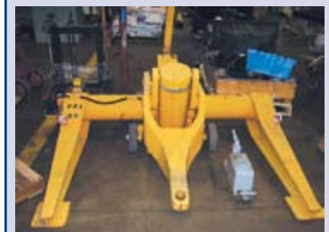
(2) Rhino 45 Ton Nose Wheel Jacks, Air Over hydraulic
