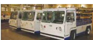
(2) Tug Mdl MH 50-1 High Speed 5000 lb DBP Tug, Perkins Diesel, Auto Trans
