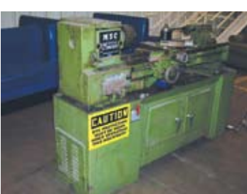
MSC Mdl 1340 CU Engine Lathe 12" Swing, 48" Gap Bed, 1 1/2 Hollow Spindle
