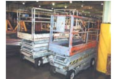
SkyJack Mdl 5J 3220 Scissor Lift, 500 lb Cap, 20' Lift SkyJack Mdl SJ4626 Scissor Lift, 800 lb Cap, 26' Lift
