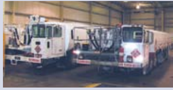
DART 10,000 Gal Low Profile Jet A Truck, 1 Sided Single Point Nozzle, 2 Under Wing Single Point Nozzles, Bottom & Top Load, Fuel/Defuel Capable, Facet Filter System, Detroit Diesel Engine, Brown Stainless Steel Tank
