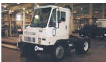
1995 Ottawa Mdl 4T30 Yard Tractor w/Cummins Diesel Engine & Allison Transmission
