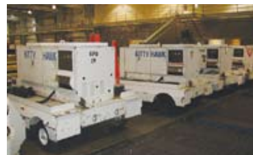
(12) Hobart Mdl 90G-20P GPU'S, 90 KVA, Detroit Diesel Engine (3) Hobart Mdl 90P20P GPU'S, 90KVA, Perkin's Diesel Engine (2) Hobart Mdl 90GT20P GPU, 90 KVA, John Deere Diesel Engine (5) Hobart Mdl 60-G20P GPU'S, 60 KVA, Detroit Diesel Engines Hobart Mdl 60P20P GPU, 60 KVA, Perkins Diesel Engine
