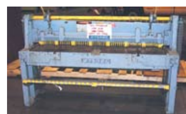
Wysong Mdl 1672 6' Sheet Metal Shear, 16 Gauge Cap
