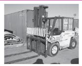
Hyster MdI H155XL2 Forklift, 15,000 Lb, 24' Triple Stage mast, Diesel Engine, Pneumatic Dual Front Tires w/Cab
