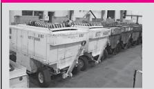
(6) USAF Type AM32A-60B Turbine Engine Driven 400 Cycle Generator Set w/Air Start Cart, Cap 75 KVA, 3 PH, 400 Cyl, 120/208 Volt AC, 500 Amp, 30 Volt DC, Pneumatic 120 Lbs Per Min @ 49 PSI, Mfg By Libby Welding Mdl LGT-60, Has Aireasearch Mdl GTC-85-
