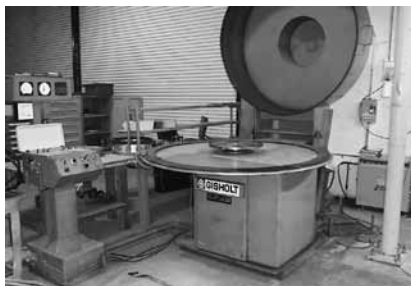
Gisholt Type SV-250 Static Vertical Balancing Machine, Serial # 4649x2, 54" Max Rotor, Manual Controls, w/ GE Mdl. 6V10F3095X SCR Speed Variator For 10 HP Motor
