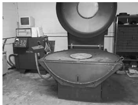
Schenck Mdl VE4L Static Vertical Balancing Machine, Serial # AVF8517, Mfd. 1999, Weight Range 5-330lbs, 120-5000 RPM, Shroud Inside Diameter 62", Balancing Accuracy 30 Micro-Inches or Better, 15 HP Drive Motor, w/Schenck CAB690 Control Head and Computer Monitor
