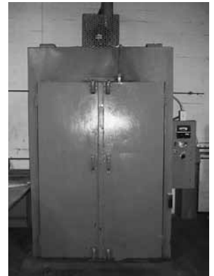
Gruenberg Electric Company Mdl. T65V960 Cart Type Electric Oven, Serial # 3066, Max Temp 650°, 33,000 Watt, 48" Wide x 72" Tall x 48" Deep
