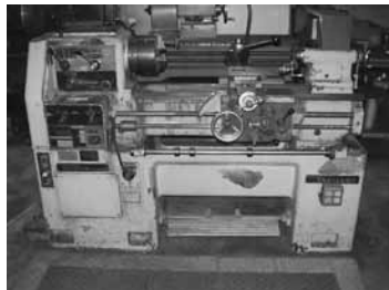
Takisawa Mdl. TSL-800 Lathe, 48" Bed, 28" Between Centers, 12" Swing, 55-1800 RPM Spindle Speed
