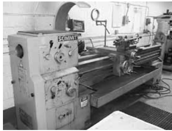
Summit Mdl. 19-4 x 80 Gap Bed Lathe, 19" Swing Over Bed, 10 3/4" Swing Over Cross Slides, 27" Swing Over Gap, 15 3/8" Gap Length, 4 1/8" Hollow Spindle. 108" Bed, 80" Between Centers, Spindle Speed 22-1500 RPM. 3 Jaw Chuck, w/Saphire DRO Counter
