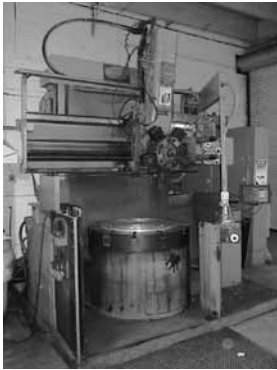
Bullard 46" Dynatrol Vertical Turret Lathe, Serial # 33390, Max Swing 58", Max Height under Cross Rail 40", Turret Swivel 30", Side Head Travels 38.75" Vertical & 23.75" Horizontal, 40 HP Motor, w/Newall DP7 Digital Readout Bullard 36" Vertical Turret Lathe, Serial # 19642
