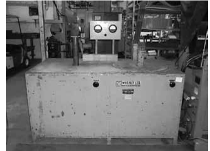
Magnaflux Type X2152 Post Type Magnetic Particle Inspection Bench Magnaflux Type SB-2814 AC Unit DeMag Bench Magnaflux Type SB-1416 DeMag Ring
