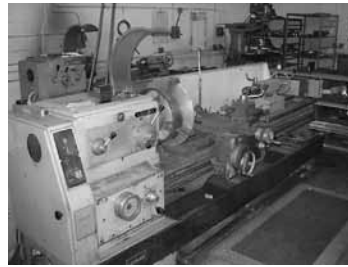
Longem Mdl. LG2080D Gap Bed Lathe, 20" Swing Over Bed, 25" Swing in Gap, 108" Bed, 80" Between Centers, 3" Hollow Spindle, 11.2-1600 RPM Spindle Speed, 4 Jaw and 3 Jaw Chucks
