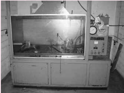
Bauer Mdl. BMI-1378 Oil Flow Test Stand (for Oil Nozzles.) w/ Cox Series 4000 Digital Flow Computer
