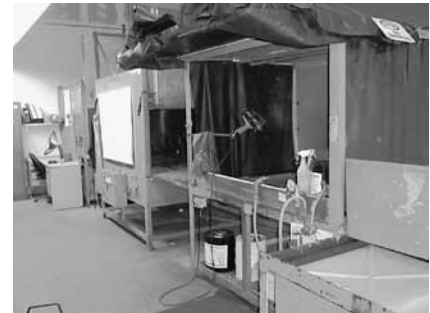
Zyglo Dye Penetrant Inspection Line, Approx 24ft. Includes Penetrant & Rinse Station, Zyglo Mdl. ZD3072S Oven, and Zyglo Developer Station. Zyglo Blacklight Inspection Booth Magnaflux ED-1500 Eddy Current Tester
