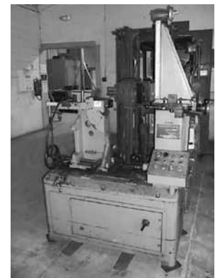
Advance Manufacturing Co Mdl. ADTB1 Universal Tab Bending Rivet Flaring Machine. Disc Diameter Swing 9.5" Minimum - 42.5" Maximum, Bed Travel 1.5" Min - 42.5" Max
