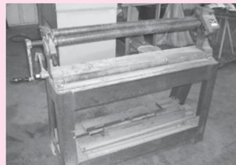
**Pexto Mdl 0381-D Sheet Metal Roller; 42" Cap, 24 Gauge Soft Steel**
