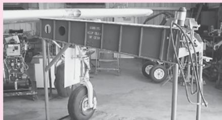
Hyd L/G Systems Trainer; Built w/Piper M/G & Wing Section, Fully Operable
