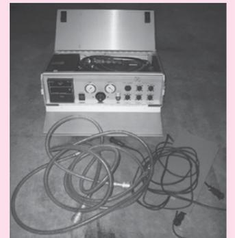
**(4) CES MDL 1000S Composite Hot Patch Complete Bonding Machines
