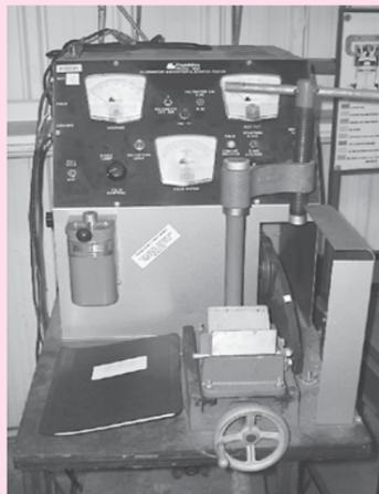
**Crumbliss Mdl 1850 Alternator, Generator & Starter Test Stand
