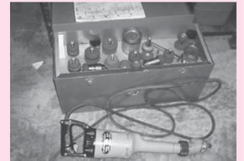
**Sioux Mdl 1695-S Angle Head Valve Seat Driver Set w/ Dresser, Pilots & Stones**
