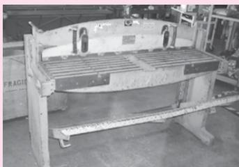
**Pexto Mdl 152-K Sheet Metal Shear; 52", Cap, 16 Gauge Soft Steel w/Back Gauge**
