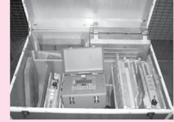
**Evergreen Mdl 2-0266-L Roadrunner Electronic Aircraft Scale w/2 ea 6000 Lb Main Wheel Scales & 2500 Lb Nose Wheel Scale**
