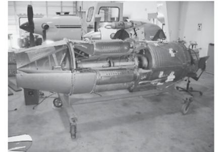
Turbine Cutaway Engine
