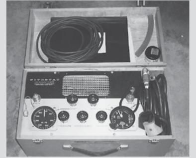
QED Mdl 5K Series Pitot Static Test Set
