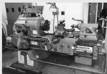
Monarch Lathe 19" Swing, 53" Bed, 30" Between Centers
