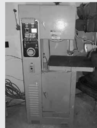
Vertical Band Saw, 14" Throat, 21"x 20" Table w/Blade Welder
