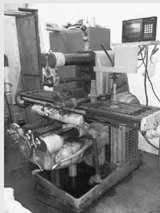
Kearney & Trecker Mdl. H, No. 3 Universal Horizontal Milling Machine, 13"x 64" Table. Has Anilam Wizard 800 Digital X Y Z Readout, 20 RPM to 1000 RPM Spindle Speed
