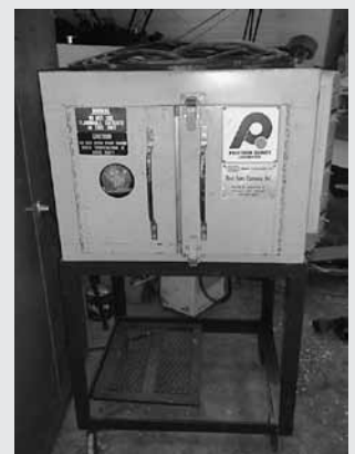
Precision Quincy Mdl. 51-1000 Electric Oven up to 900 degrees F
