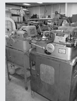
Sioux Mdl. 645L Valve Grinding Machine w/Rocker Arm Attch.
