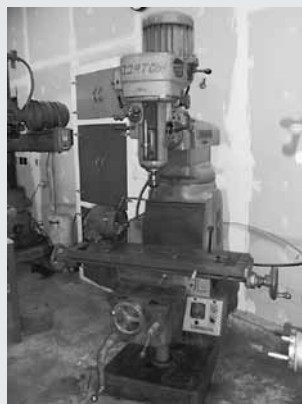
(2) Gorton Mdl. 1-22 Mastermill Vertical Milling Machines, S/N 39460 & S/N 39453 Spindle Speed 80-560 RPM Low & 800-5600 RPM High, 2-HP Motor, 42" x 10" 3 Slot Tables, Both have Dyna Drive Table Feed Units S/N 39460, Has Mitutoyo Digmatic XY DRO
