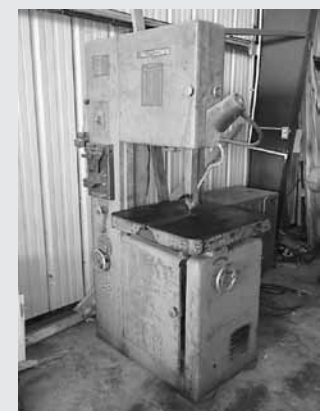
Powermatic Mdl 87 Vertical Band Saw, 19" Throat, 24" x 24" Table w/Blade Welder
