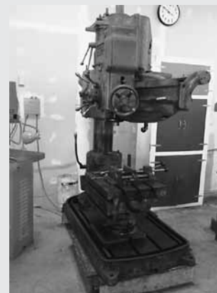
Cincinnati Gilbert Radial Arm Drill Machine #4918, Spindle Speed 50-1800 RPM, 44" Arm
