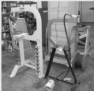
Central Machinery Mdl. 95359 English Wheel Kit & Stand 28" Throat
