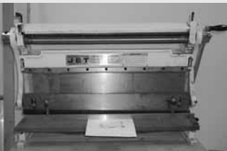
Jet Mdl. SBR-30N 3 in 1 Machine Combination Shear, Brake & Roll 20 Ga, 30"
