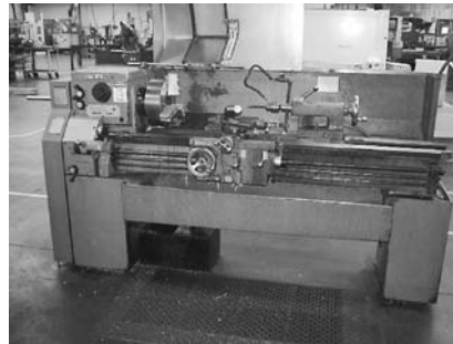
LeBlond Regal Mdl 15" Engine Lathe Servo Shift, S/N 13C-295, 5'6" Bed Length, 15-1/2" Swing Over Bed, 9-1/2" Swing Over Cross Slide, High Low Speed Range 30 RPM to 1,800 RPM, Distance Between Centers 30".
