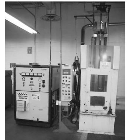
Lepel Induction Heater Mdl T-40-3-KC-E-XW, S/N 7001, 92 KVA, Durant 6460 Sequence Controller, Quench Tank, Single Station Vertical Shaft up to 92"
