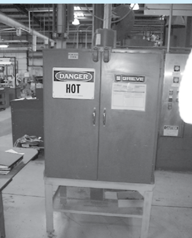
TSI Bottom Load Retort Furnace Heating Element Rating 100 KW, Max Operating Temp 2200° F, Size 40" Diameter x 40" High, Loading Capacity 1,000 LB/3 Hours, Honeywell Control Panel w/Honeywell DR-4500A Truline Circular Chart Recorder & Honeywell UDC 2000 Universal Digital Controller, Honeywell DPR Strip Chart Recorder, Gas Flow 275-300 CFH
