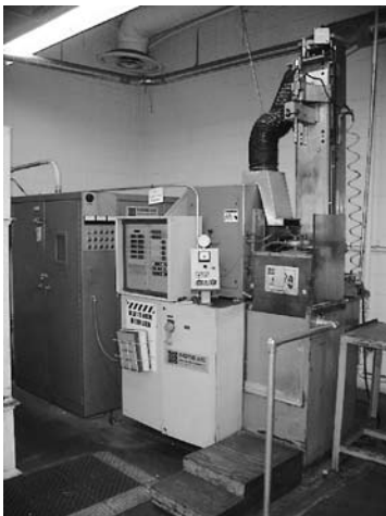
Radyne/AKO Induction Heater Mdl EI-30, S/N 110331, 30 KW-440 KHZ, Dual Station Vertical Shaft up to 36", Quench Tank, Radyne/AKO Scanner Control System
