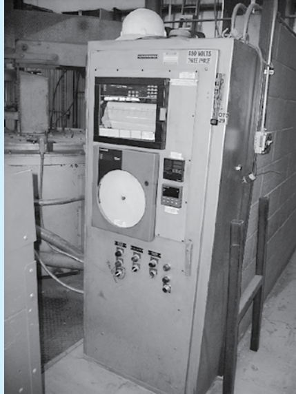
Lindberg Mdl 12-RP-4848-18A Pit Furnace S/N 24485, Max Temp 1850° F, Heating Chamber 48" Diameter x 48" High, Total Load 2,000 Lb. Lindberg Control Panel w/Honeywell LCD Readout, Chart Recorder & Honeywell Truline DR-4500A Circular Chart Recorder.
