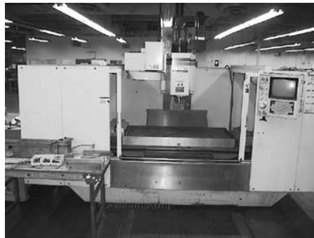
Fadal Mdl VMC-6030 HT CNC Vertical Machining Center, S/N 9208503, Has Fadal CNC-88 Control Unit, Table Size 30" x 62.5", Travels X Axis 60", Y Axis 30", Z Axis 30", Spindle Speed 40 to 10,000 RMP, Spindle Tapper No. 40, Main Motor 22.5 HP
