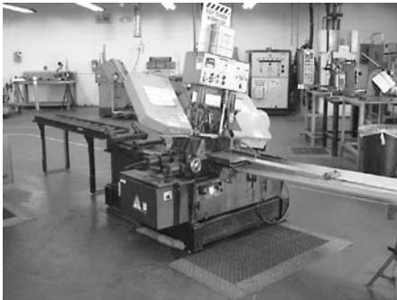
Amada Mdl HA-250 Automatic Horizontal Band Saw, S/N 25400-68, 3 HP Saw Blade Motor, Cutting Capacity Round 9.84", Rectangular 11.02" x 9.84", Speed 88 to 262 Ft/Min
