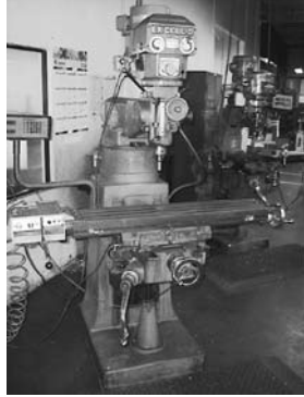
Ex-Cello Mdl 602 Vertical Milling Machine S/N 6028352, 1-1/2" HP, 46" x 9" 3-Slot Table, Spindle Speed 85 RPM to 4,000 RPM, Lyman Mdl MK-7 Power Feed Table Attachment, Has 5-1/2" Riser Block, Bridgeport 1812064 DRO.
