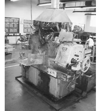
(5) Cincinnati Milacron #2 Centerless Grinding Machines, Mdl OM's, Hyd Grinding Wheel Dresser, Capacity Short Work 1/16" to 3-1/2" Diameter, Bar Work 1/8" to 2" Diameter.
