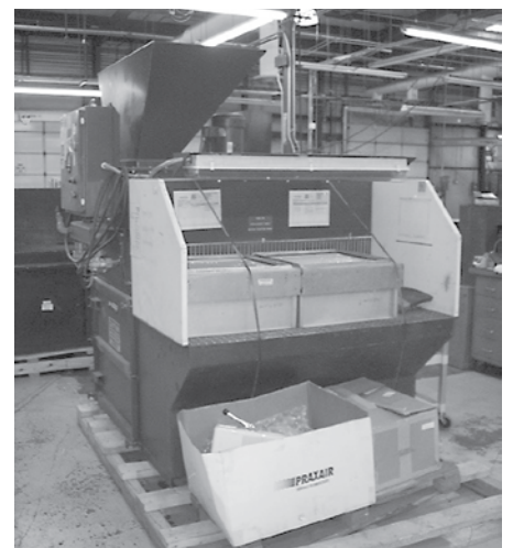
Uni-Wash/Polaris Mdl V-4000 Down Draft Blending Booth, 5' Wide Donaldson Torritt Mdl VS-1200 Dust Collector, 3 HP
